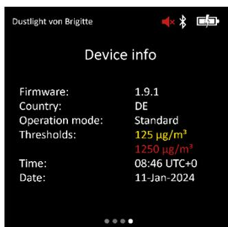
The last screen displays device information, including the software version of the Dustlight, the country in which the Dustlight is operated and its applicable limit values for the particulate matter content of the air, which are automatically adopted via the app. The UTC time and date of the device are also displayed. If these deviates too much from the actual time, please synchronize your Dustlight via the app. The values are displayed in the app in your correct time zone.
