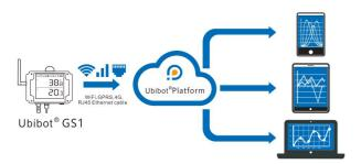
The GS1 continuously monitors environmental conditions and syncs the data to the UbiBot®IoT Platform. By offering 4 ways of data transmission, it can ensure different users access the online data using our App or the website.
